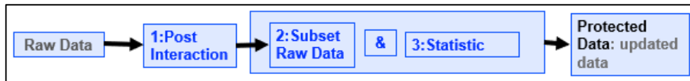
Figure 2.4: Noise Inclusion Order Used by Randomization Privacy Mechanism to Produce Protected Data; Updated Data. 1: When to Add Noise, 2: Where to Add Noise 3: What Noise to Add.
