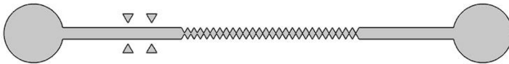
Figure 4. Schematic showing the top view showing the microfluidic apparatus used in insulator based DEP. The device is roughly 4 cm in length with 24 teeth like structures constructed of PDMS with the largest teeth gap being 30 \mu m and the smallest being 3 \mu m.
