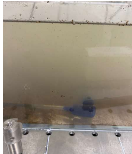
Figure 5.13: Side view of the water tank after adding the milk and sand.
