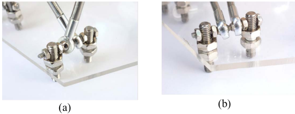
Figure 18. Rod end bearing which enables smooth rotation.
