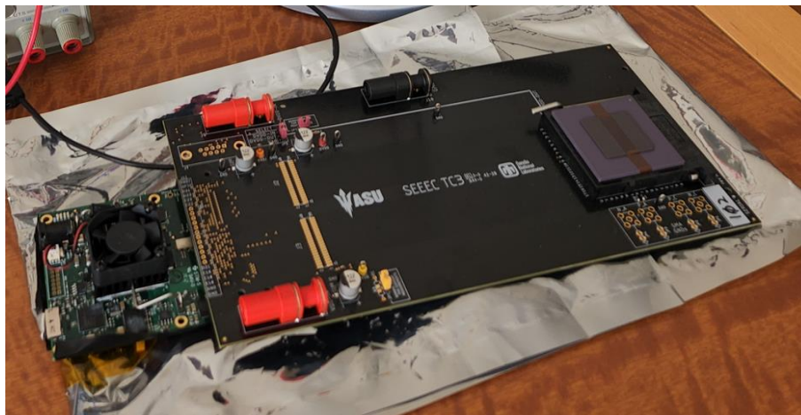
Figure 5.1 Packaged part socketed into the daughter card and connected to the Xilinx FPGA controller.
