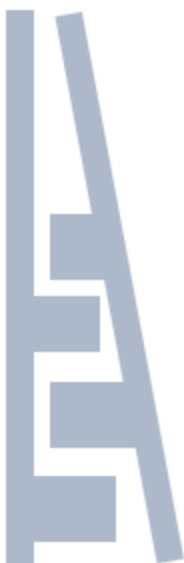
Figure 4.12 Cut pattern to measure parasitic capacitance of the rolled inductor.
