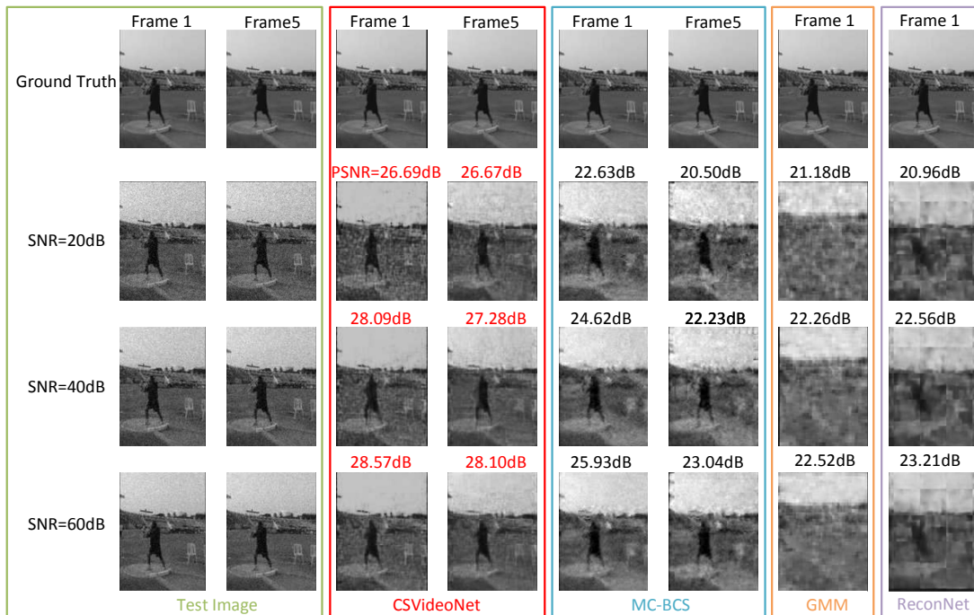
Figure B.2: Reconstruction result for each algorithm at the CR of 25 when inputs are contaminated by Gaussian white noise with the SNRs of 20dB, 40dB and 60dB.
