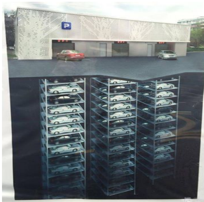
Figure 13: Yicheng Underground Parking (Weiyuan, Z. 2020)
