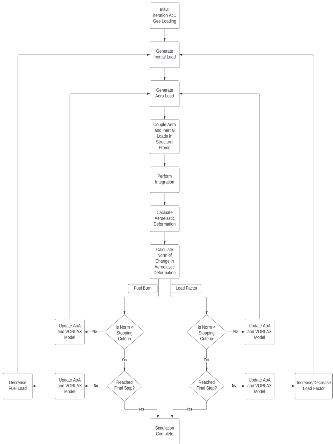
Figure 35. Load Factor and Constant C_L Fuel Burn Solution Procedure.
