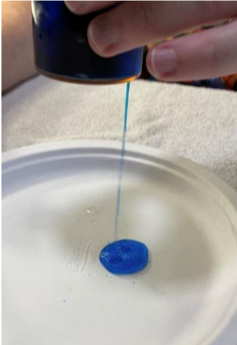
Figure 21. Photograph demonstrating the functionality of the overflow tube. Note the blue liquid represents excess urine from the MSCC specimen.
