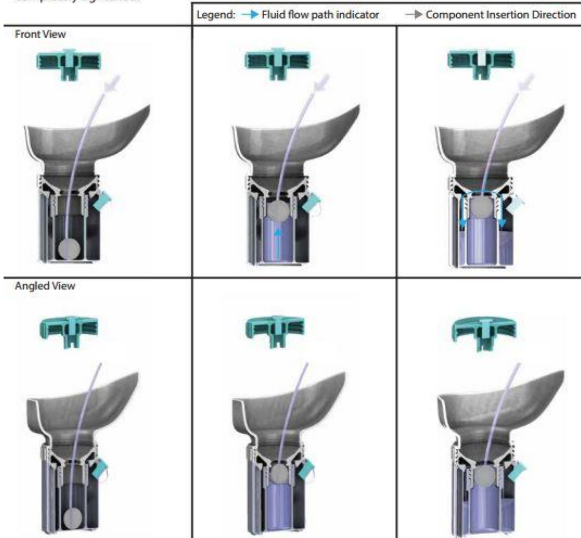
Figure 17. Storyboard rendering demonstrating the fluid flow and device operation during the fill phase.
