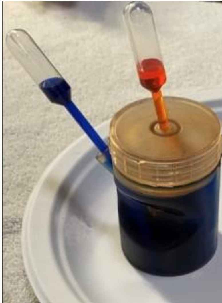
Figure 20. Photograph of the prototype device during the extraction phase. The blue sample is the MSCC portion and the red sample is the initial void sample. Note if they had mixed, one or both samples would be green.
