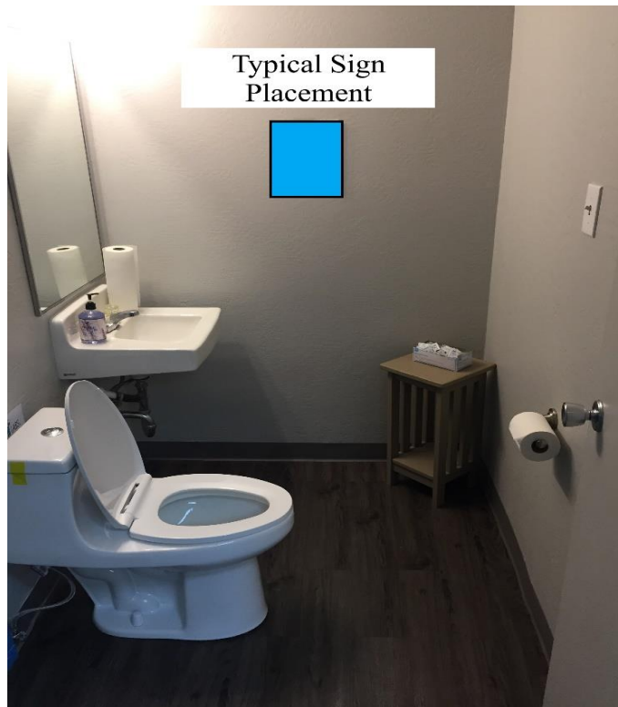
Figure 5. MSCC typical sign placement. Single sign placed so that men can see it to their right while standing and women can see it to their left while sitting.
