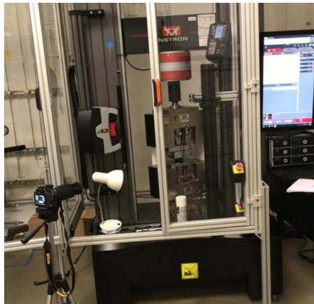
Figure 33 : Compression Testing Setup
