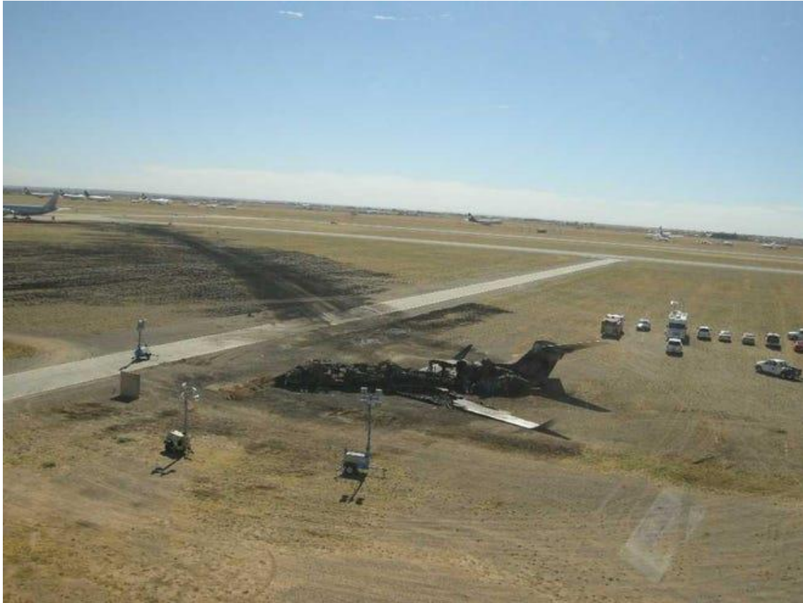
Figure 3. Remains of the flight-test Gulfstream G650 after pilots continued takeoff with an in-ground-effect stalled wing [5]
