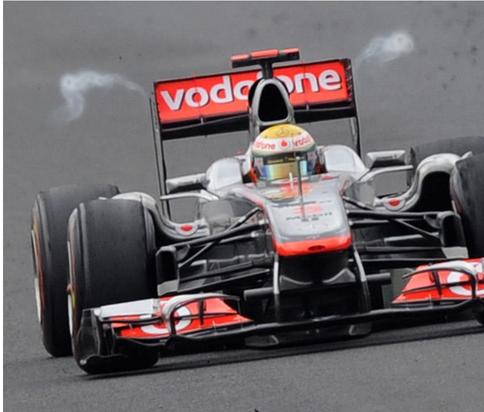
Figure 8. Picture of an F1 car where wing tip vortices are visible [24]
