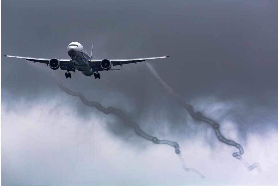
Figure 7. Picture of a commercial aircraft where wing tip vortices are visible [23]
