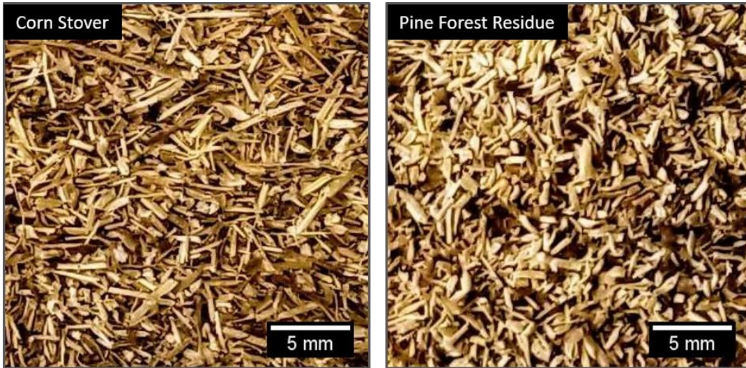
Figure A. 1. Corn stover and pine forest residue fines produced from hammer milling
