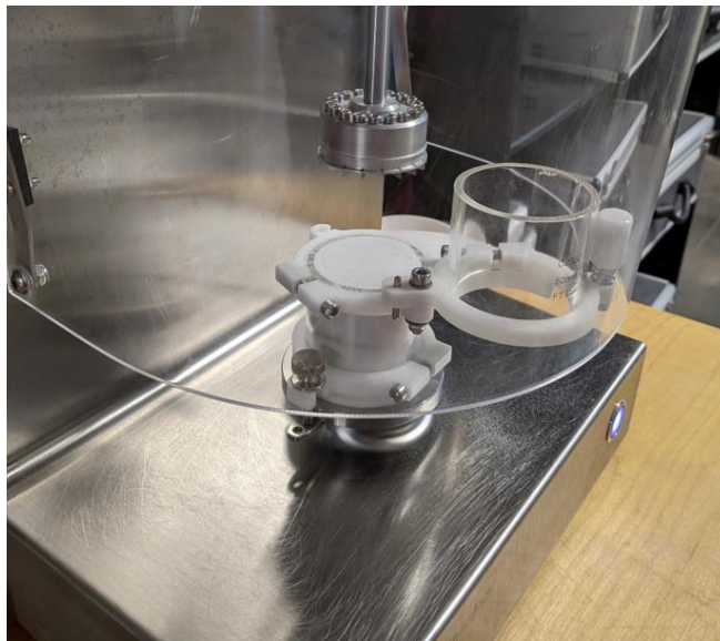
Figure 7. The vessel used for the shear cell test on the FT4. The splitting mechanism is used to get rid of the excess material, resulting in and we are left with a flat surface for the experiment.
