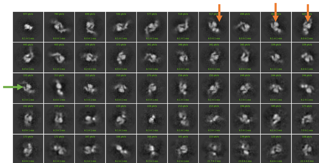
Figure 4.4. Two-dimensional classification of \alpha\beta 8 -pro-TGF \beta 1 . Different orientations of the complex were represented in orange arrow, and the unbound integrin was represented in green arrow. The 2D classes were performed with k number of 50.
