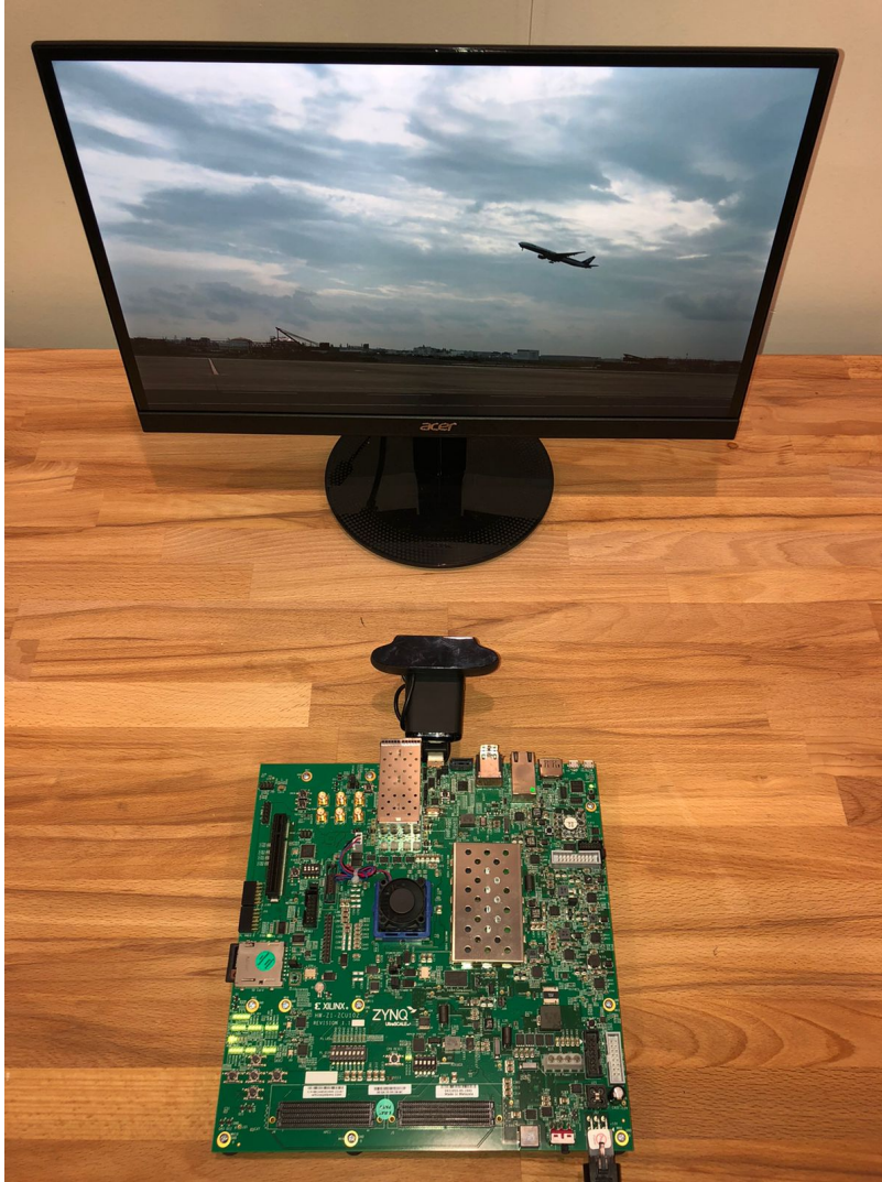
Figure 11. Our hardware setup: A sequence is displayed on an Acer LCD monitor. A Logitech C920 webcam connected to a ZCU102 board captures an image on every keyframe to perform object detection. Our system emulates ROI capture by predicting the bounding box every subsequent frame. This information would be sent to an ROI camera to perform adaptive subsampling.
