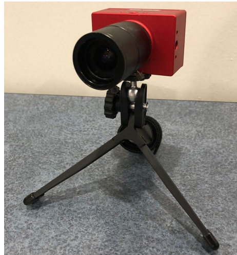
Figure 28. DAVIS 346 Event-based camera: a 346 x 260 resolution image sensor. Has the capability to capture both intensity frames and events.
