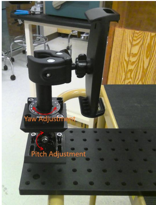
Figure 3.19: Modified Fixture for Monostatic Measurement Setup
