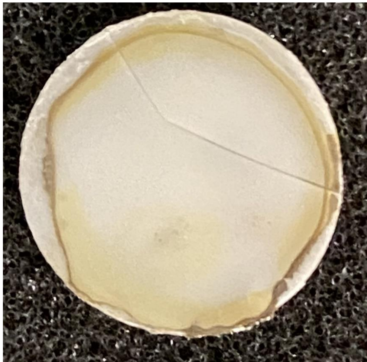
Figure 3.5 Bottom (fuel inlet) side of YSZ pellet after 48 hours H 2 +N 2 +D4 (2.5 ppm) experiment at 750 °C.
