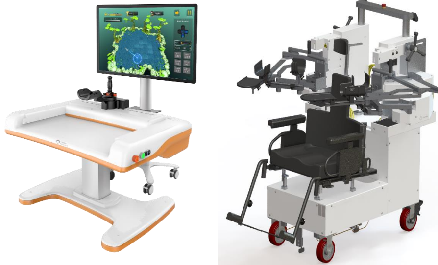
Figure 8: Fourier Intelligence ArmMotus M2 (left side) (a typical end-effector robotic device used for upper extremity stroke rehabilitation) Figure 9: Kinarm Exoskeleton (right side) (a typical exoskeleton robotic device used for upper extremity stroke rehabilitation)(Kinarm Exoskeleton Lab, n.d.)
