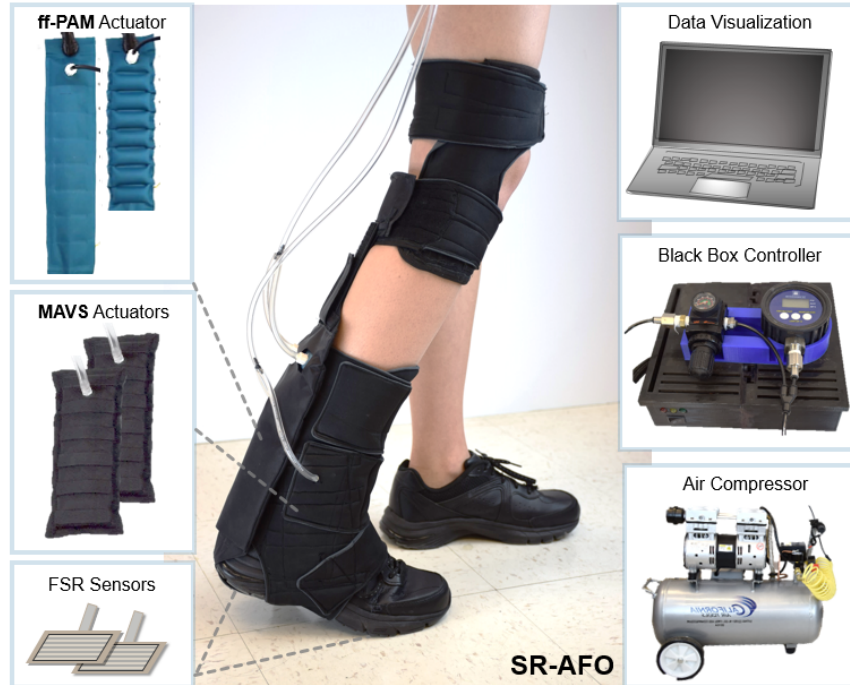
Figure 3.17: The final assembly of the SR-AFO and all components. (Left) Each actuator set and the sensors for gait detection. (Right) The controller, pneumatic source, and connection for user feedback and system information for diagnostics.
