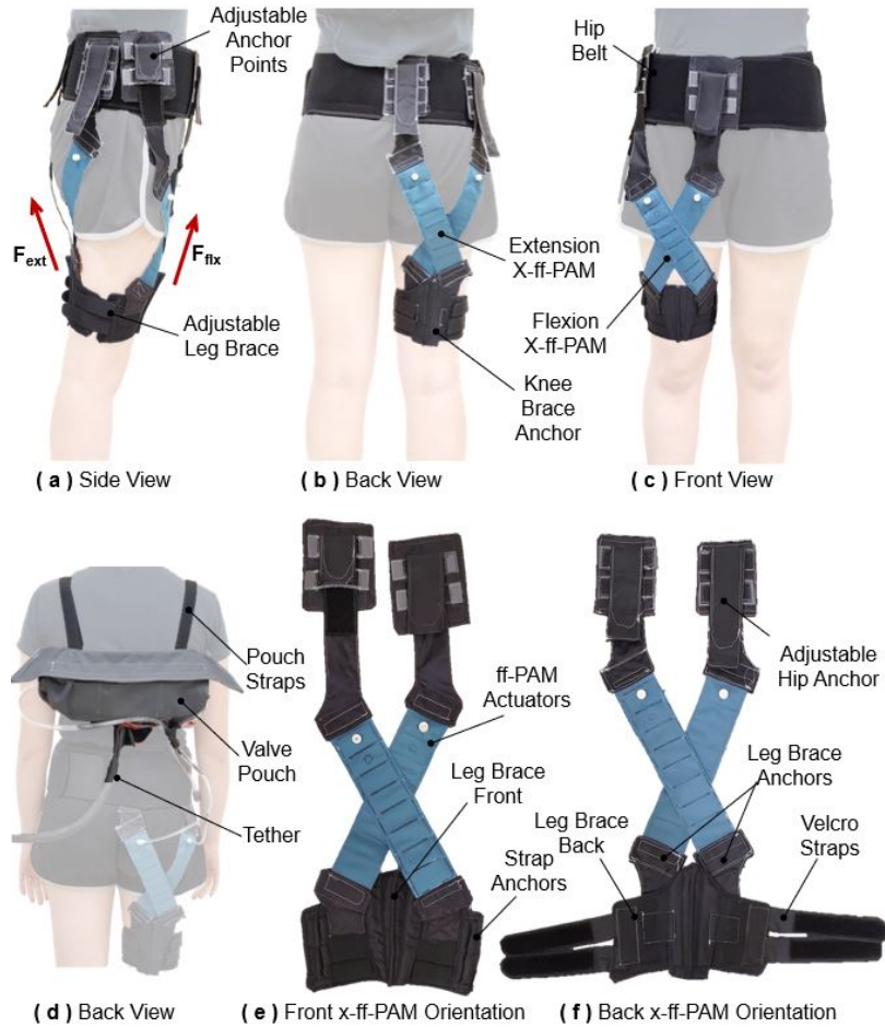
Figure 6.2: The SR-HExo shown on a user from (a) the side profile, (b) back view, (c) front view, and (d) back view. The actuator anchor points and adjustable leg brace in (a) are highly modular to fit many users. The X-ff-PAM used for actuation in flexion (e) and in extension (f) including the modular knee anchor point.
