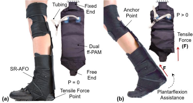
Figure 5.2: (a) A side view of the SR-AFO donned by a user in the passive condition, as well as the dual ff-PAM setup prior to inflation. (b) The SR-AFO during the active condition (inflation of the ff-PAM actuators) to assist plantarflexion.
