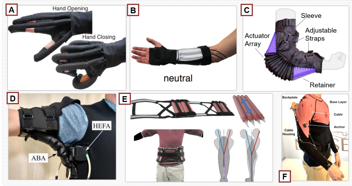
Figure 2.4: A brief survey of recent SWR technologies for each of the following upper body joints: A) a soft robotic hand developed at Harvard University at the Wyss Institute for Biologically Inspired Engineering (Cappello et al. , 2018b), B) a soft assistive device for the wrist made from fabric materials (Realmuto and Sanger, 2019), C) a soft elbow exosuit designed at Arizona State University (Thalman et al. , 2018), D) Shoulder assistive device also from Harvard University at the Wyss Institute for Biologically Inspired Engineering (O’Neill et al. , 2017), E) Trunk Orthosis from the Reconfigurable Robotics Lab at Ecole Polytechnique Fédérale de Lausanne (Robertson, 2019; Robertson and Paik, 2016), and F) an upper body device that assists multiple joints via cable-driven actuation (Lessard, 2018)
