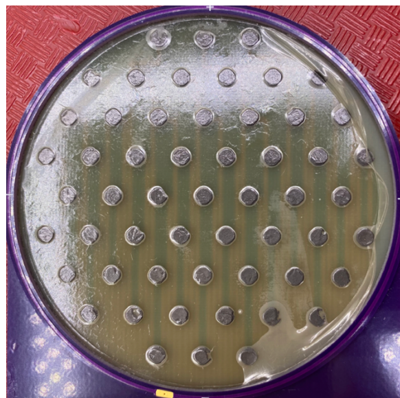
Figure 42 - Photo of Post-Experiment Peeling Due to Drying Out.
