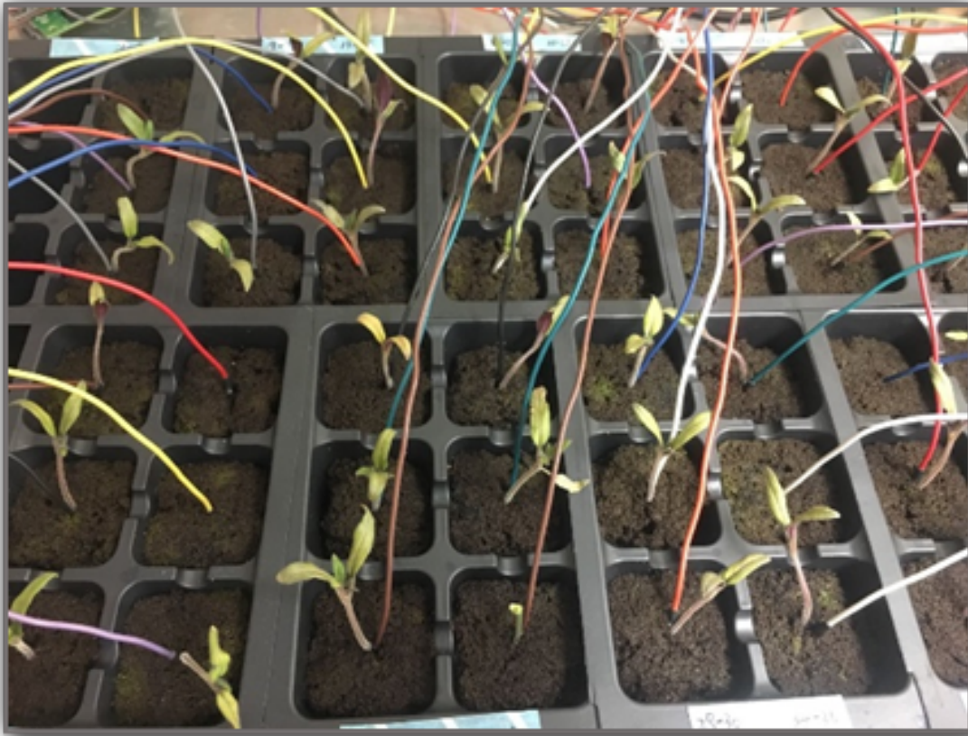
Figure 17 - Seeded and Unseeded Coated and Uncoated Probes in Randomized Tray Experiment (Qi, 2021)
