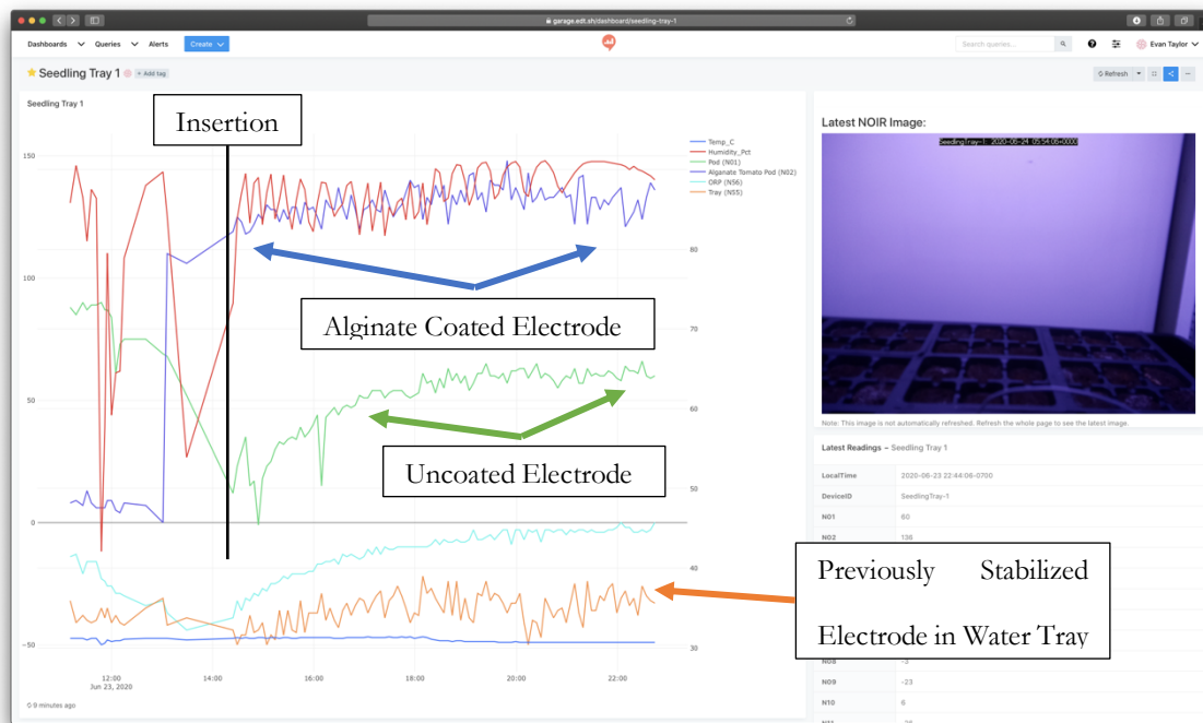
Figure 15 - Initial Testing of Alginate Coated Electrodes in a Hydroponic Seeding Tray.
