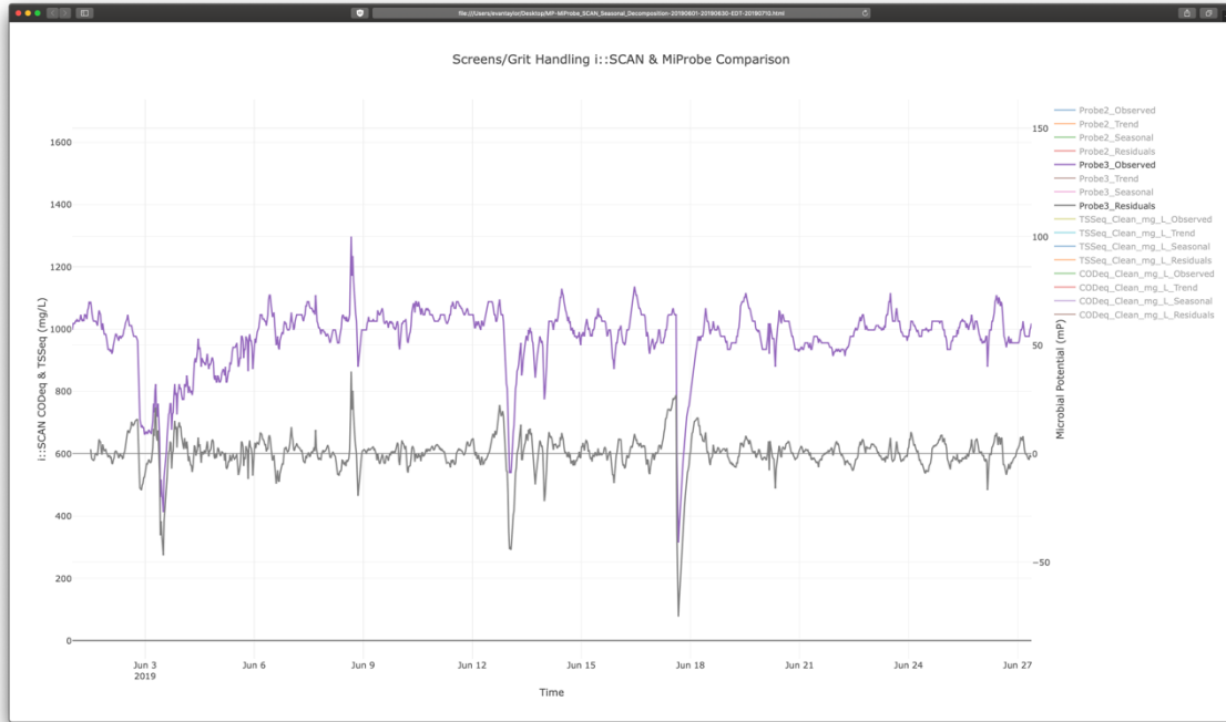
Figure 6 - Comparison of Observed and Decomposed Residuals of MiProbe Sensor Data from a Wastewater Treatment Plant.
