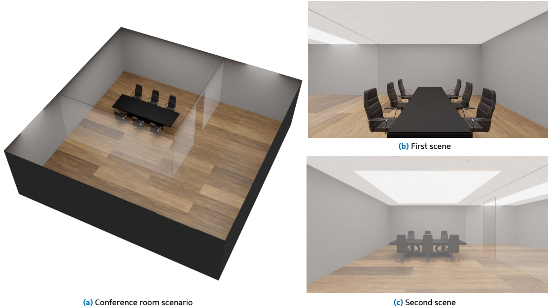
Figure 3.24: (a) the Bird View of the Conference Room Scenario; (b) and (c) the Scenes under Study. The 10\text{m} \times 10\text{m} Indoor Space Contain a 6\text{m} \times 6\text{m} Conference Room in Glass. The Indoor Space Walls Are Made from Layered Drywall, the Ceiling Is Made from Ceiling Board and the Floor Is Made from Floorboard. The Conference Room Chairs and Tables Are Made from Wood.
