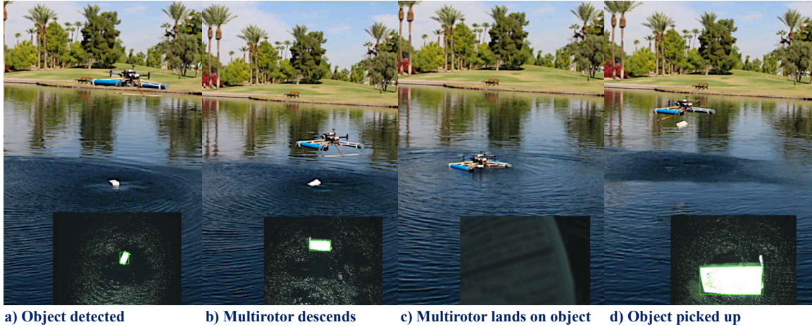
Figure 15: Successful collection of an object from water surface by the multirotor specularity removal algorithm has decreased the contrast of the background water surface by a lot, while also highlighting the features of the object. However, failure cases were seen when testing dark can. Since the video collected using the dark can was during a cloudy illumination condition, the edges object had low visibility, as the background was also quite dark. In addition to this, using the polarization filter and the specularity removal algorithm reduces the contrast of the image, which also resulted in the dark can being masked by the background in a number of frames. While the detector does not through any false positives, it failed to detect the object for a number of frames and reverted back to estimation even though the object was in the frame. This caused a decrease in the number of successful collection of the dark can by the multirotor.
