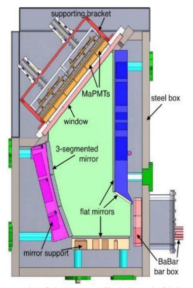
**Figure 2.17:** Cross section of photon camera. The BaBar pads slide into the bottom and the light is bounced into the MaPMT.
