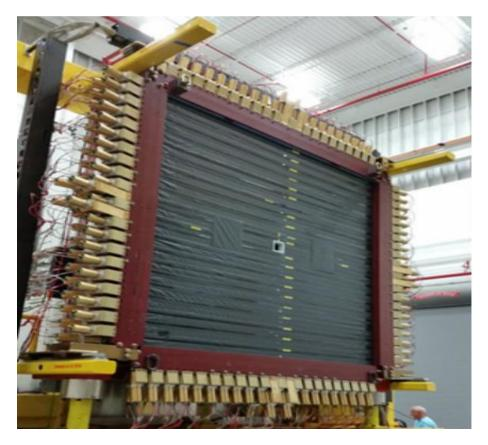
Figure 2.15: A fully constructed TOF Detector with a  $12x12 \text{ cm}^2$  cutout for the beamline.
