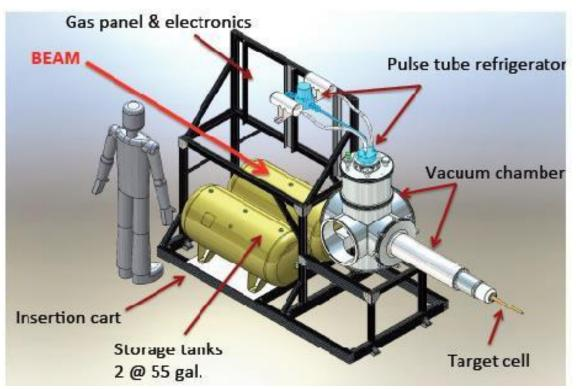
**Figure 2.9:** Pulse tube refrigeration system, comprised of a pulse tube refrigerator, vacuum chamber, two safety storage tanks, and the target cell filled with  $LH_2$ .
