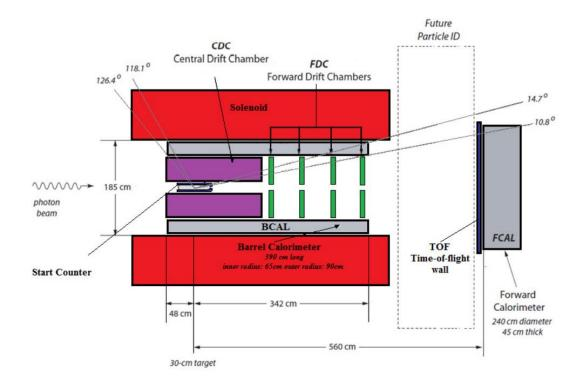
Figure 5.6: Illustration of the GlueX Spectrometer with polar acceptance angles.
