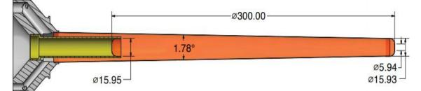
Figure 2.8: Diagram of conical target with dimensions given in degrees and inches.
