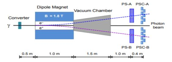
**Figure 2.7:** Illustration of the pair spectrometer. The photon beam comes in from the left and is incident on the converter that is common to both the TPOL and PS. When pairs are produced in the convertor, those pairs enter the PS magnetic field and then move through the vacuum chamber and finally to the detector elements. The detector elements are shown as PS and PSC, where the PSC are course counters.
