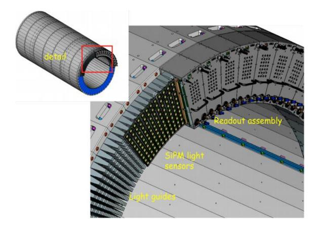
Figure 2.14: 3-D model of BCAL readout system, showing the light guides, silicon photomultipliers and the readout system.
