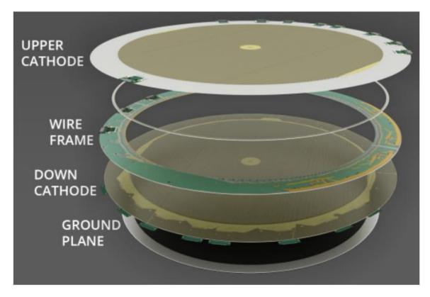
**Figure 2.13:** Individual FDC package. From bottom to top, the FDC package starts with a ground plane followed by a down cathode, wire frame assembly and topped off with an upper cathode layer.
