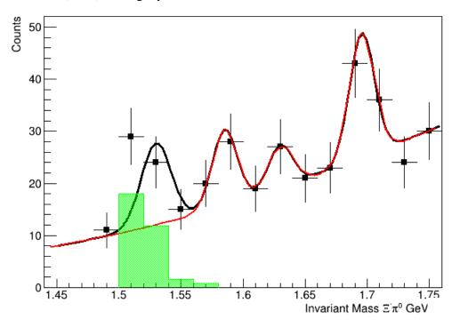
**Figure 8.10:** Invariant Mass Distribution of  $\Xi^{*-}$  in GeV with  $\cos\theta_{GJ}$ , between 0.6 and 0.8, with extracted  $\Xi(1530)$  having a yield of  $32 \pm 6$ .
