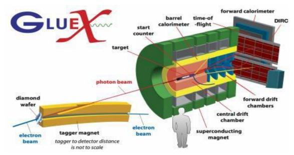
**Figure 2.6:** A compactified graphical representation of the Hall-D experiment from photon tagger to the GlueX spectrometer, and finally the forward detectors.
