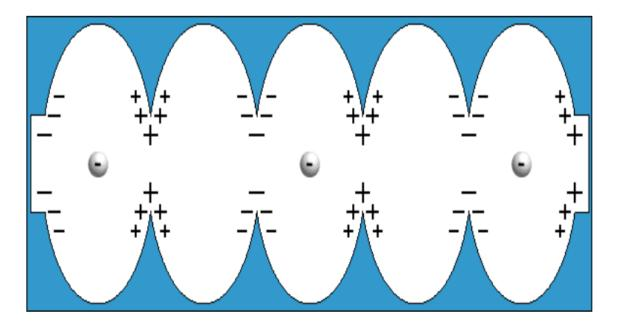
**Figure 2.2:** Illustration of the cavities used in Hall-D, the polarity is flipped each time the electrons travel to another node in the cavity in order to accelerate the electrons through the space.
