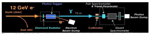
**Figure 2.3:** Hall-D Beamline beginning from the linearly accelerated electron beam passing through the photon tagger into the GlueX spectrometer and finally into the beam dump.
