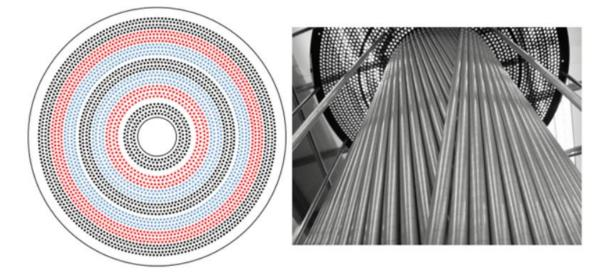
**Figure 2.11:** The CDC endcap straw-tubes layout is shown on the left, and the CDC partially filled with straw tubes is on the right.
