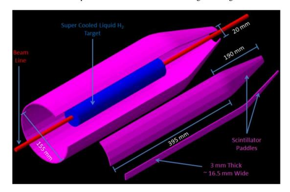
Figure 2.10: Drawing of start counter surrounding  $LH_2$  target, tapering toward the beamline on the downstream side.
