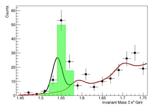
**Figure 8.11:** Invariant Mass Distribution of  $\Xi^{*-}$  in GeV with  $\cos\theta_{GJ}$ , between 0.8 and 1.0, with extracted  $\Xi(1530)$  having a yield of 78  $\pm$  9.
