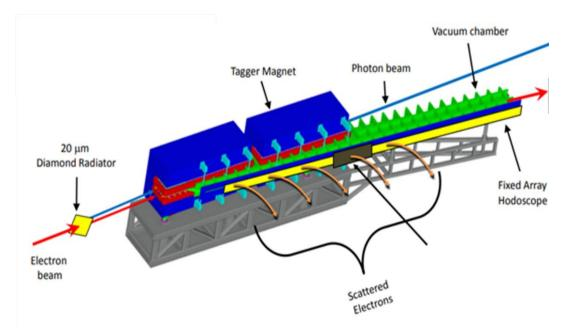
**Figure 2.4:** Depiction of the electron beam incident on the diamond wafer entering the tagger microscope and hodoscope.
