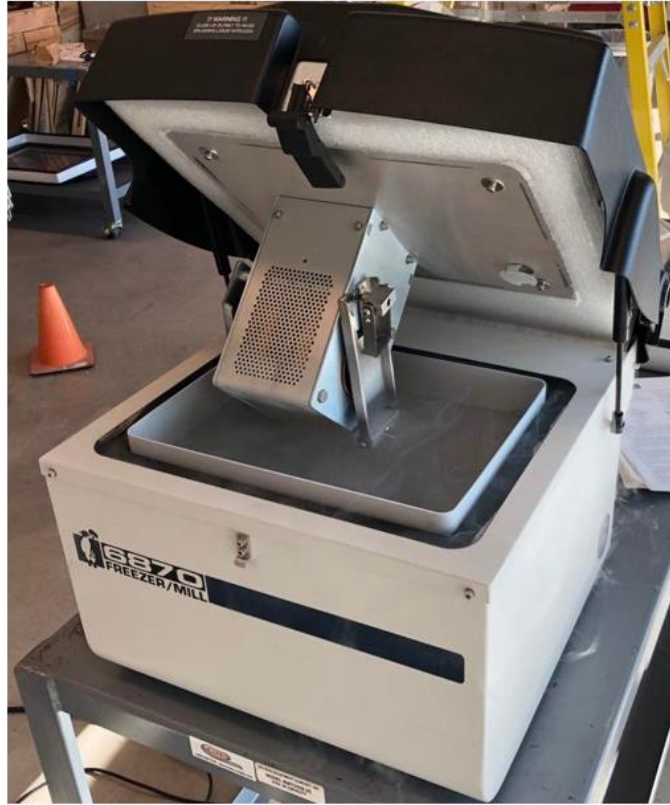
Figure 51 – Cryo Mill 6870 to Reduce Particle Size
