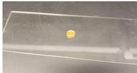
Figure 17: 10 \mu L of the beads placed as a droplet on a glass slide. The glass slide is approximately 25 mm x 75 mm, the standard size for microscope slides.
