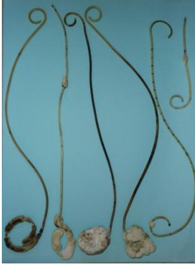
Figure 2.5 Example of severe encrustation on a polyurethane ureteral stent. These stents require surgical removal, a costly and dangerous procedure for the patient. 67
