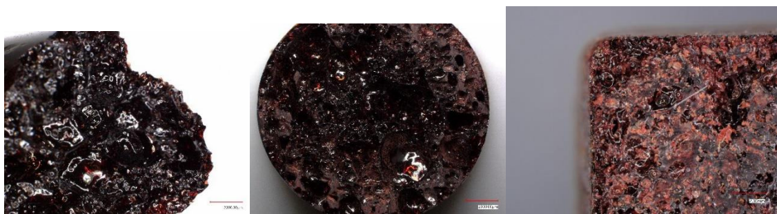
Figure 9.4: Microscopy of molded foam cross sections reveal good shape retention and closed cell structure. The addition of a Michael acceptor to the BCI formulation resulted in increased gloss of the final part.
