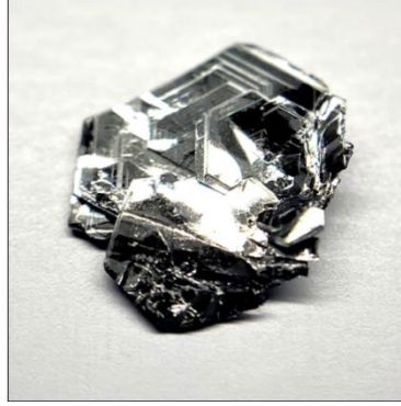
Fig 2. 1 WSe 2 bulk crystal-synthesized via chemical vapor transport © 2D semiconductors.
