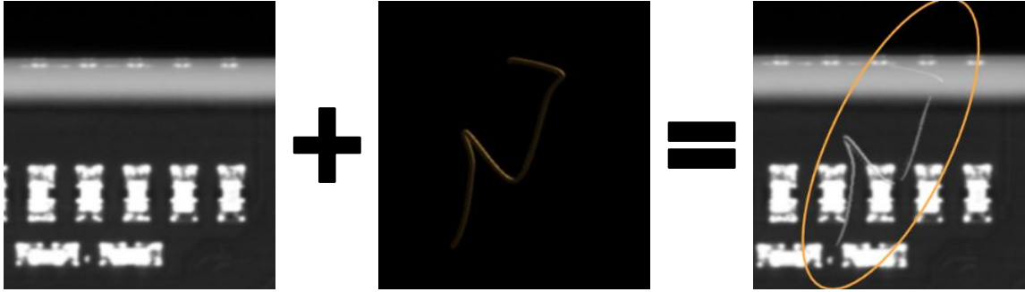
Figure 3.6: Example of Alpha Blending. Left Image Is the Non-defect Sample, Middle Image Is the Rendered FM Image, and Right Image Is the Blended Image.
