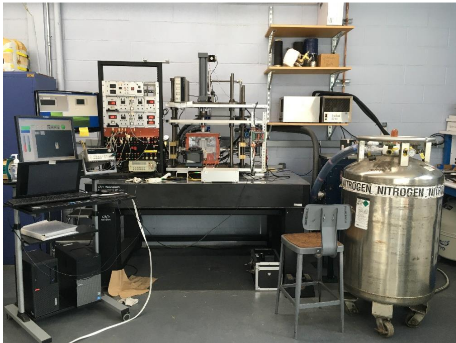
Figure A.2: Biaxial cryogenic deformation apparatus at LDEO (pictured above) is used with LN to achieve cryogenic temperatures and simulate a broad range of velocities.
