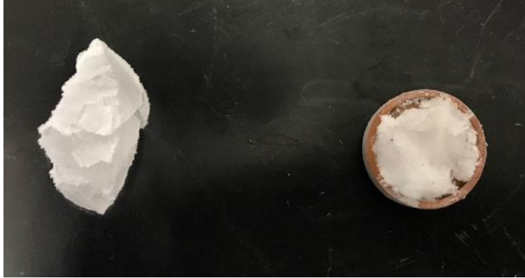
Figure 4.14: Freezer ice (FI) is ground, sieved and transferred to sample holder for the experiments in Section 4.3.1.2.
