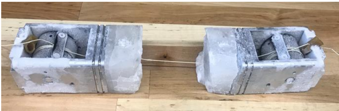
Figure 7.15: Ice Sample with STFOC tether after shear testing at \sim 230 K (brittle portion of ice shell): the central ice block is completely pulverized.
