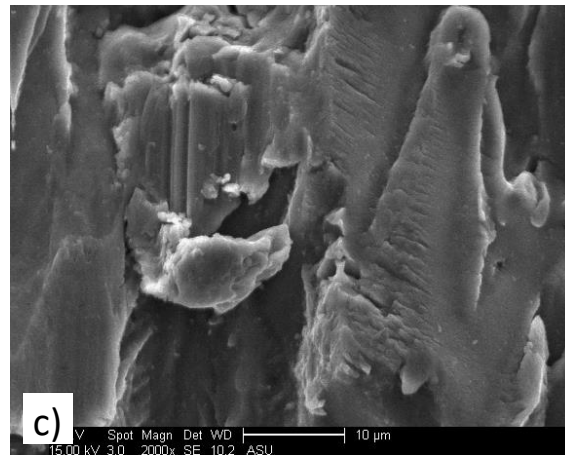
Figure 3.21: a) Microscale fracture features in the transient region of the specimen after the application of 1 st shear overload (30k cycles) with R_{OL} = (1, -1) . Magnified images of transient region showing features of shear fracture: b) cleavage steps; c) tongue and tire tracks.
