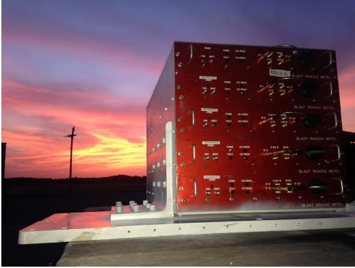
(a) The ROACH2 MOTEL , a stack of five ROACH2s which readout the five LEKID arrays for BLAST-TNG.
