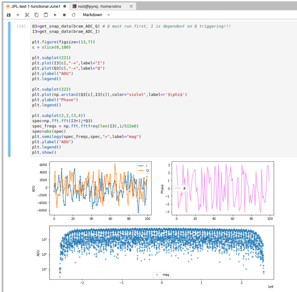
Figure 3.8: Jupyter Notebook showing it's use for grabbing data from the snap blocks and plotting. This screen grab displays the I and Q timestreams from the ADC and the spectrum computed by Python.
