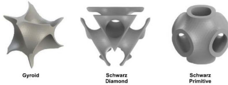
Figure 6. Unit cell visual representation of TPMS Structures (a) Gyroid structure (b) Diamond Structure and (c) Schwarz- Primitive structure [24].
