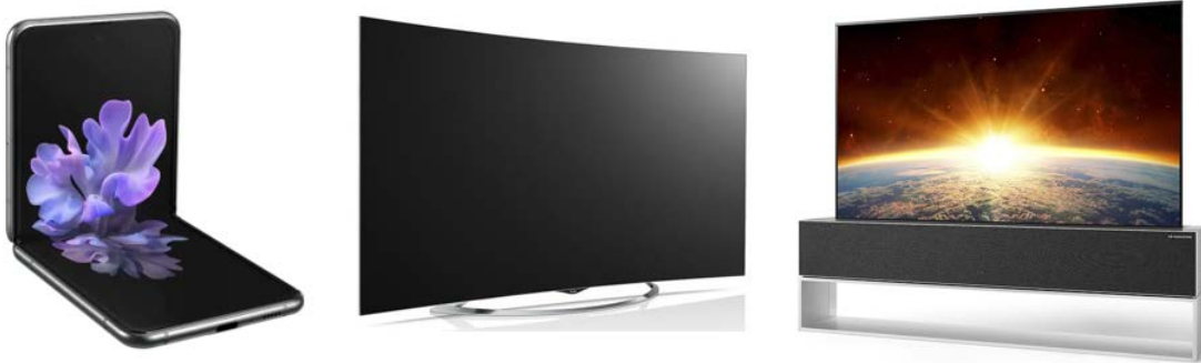
Figure 4. Personal electronics employing OLEDs. Images of Samsung foldable smartphone, LG curved television, and LG rollable television are included.
