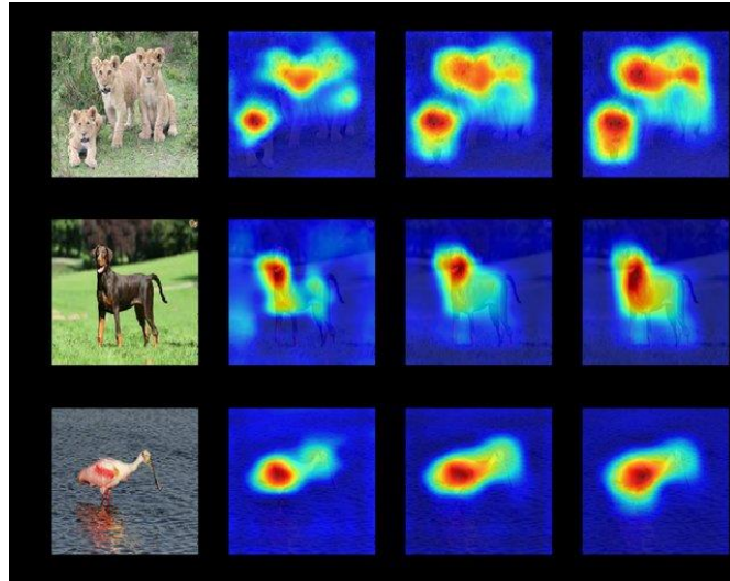
Figure 2.4 A Saliency Map. The closer to red the color, the more important the pixel for the classification of the image. Source [43] .
