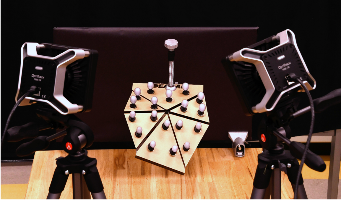
Figure 3.1: A 6-bar laminate mechanism. The experimental setup shows the use of OptiTrack cameras to record the motion of this mechanism.
