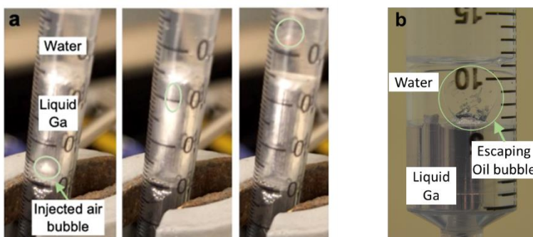
Figure 1.4 Buoyancy driven escape of injected fluids to the top surface of LM (a) air bubble, (b) Silicone oil bubble
