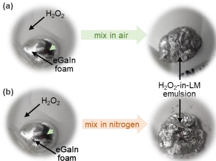
Figure S5. Mixing of LM foam with hydrogen peroxide in (a) air and in a (b) nitrogen environment
