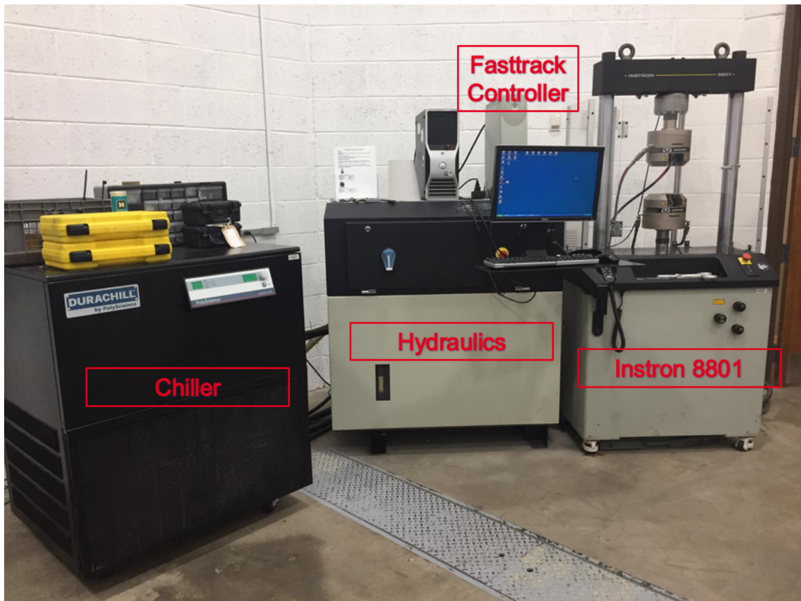
Figure D.1: Complete Fatigue Test Setup
