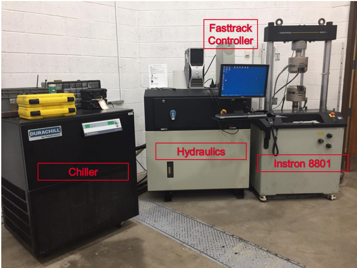
Figure 3.9: Instron 8801 Servo-hydraulic Fatigue Testing System Setup
