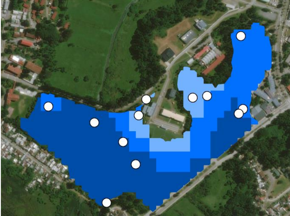
Figure 2.3. Soil sampling locations in a monitored wetland during the dry season. Color gradation from light blue to dark blue indicates increasing wetland depth, from the shallowest third of the wetland to the deepest third of the wetland.
