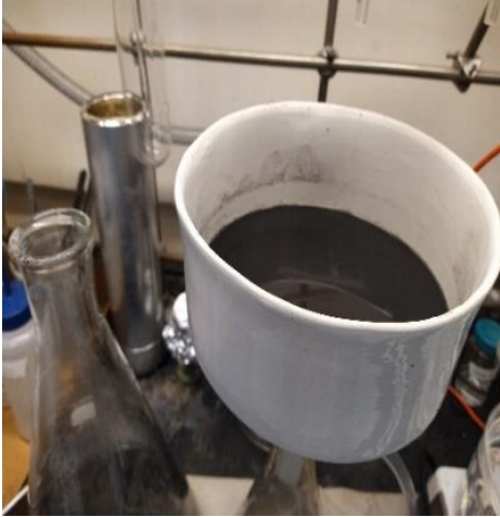
Figure 3b. Experimental set up for dissolution, filtration and reprecipitation of HDPE
