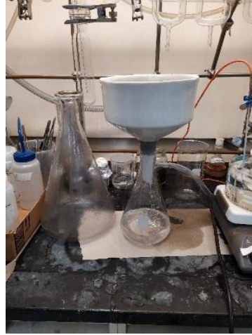
Figure 3b. Experimental set up for dissolution, filtration and reprecipitation of HDPE
