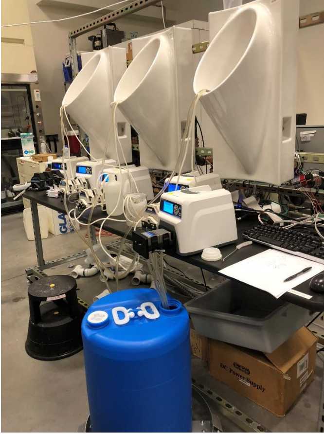
Figure 3-S10. Front of the urinal testbed. Pumps for urine, urease, and acid are on the right. Two pumps for grab samples are on the left.
