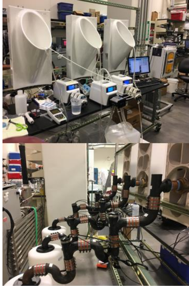
Figure 2-2. Front and back of urinal testbed. Pumps were used to deliver synthetic urine, urease solution, and acetic acid to the three urinals. The sensors were placed inside the two P-traps and in the urine storage tanks.
