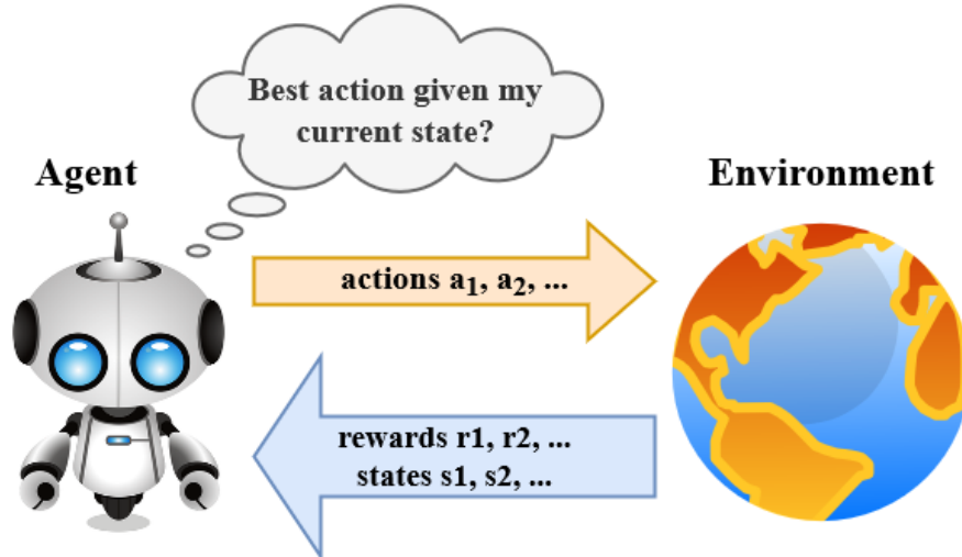
Figure 2.3: The process of reinforcement learning is to find an action decision strategy given states which rewards the agent the most in the long run.
