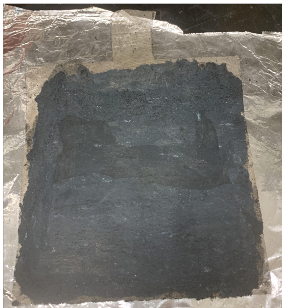
Figure 4: Image of Cathode with C-Fe-N catalyst and PTFE binder.
