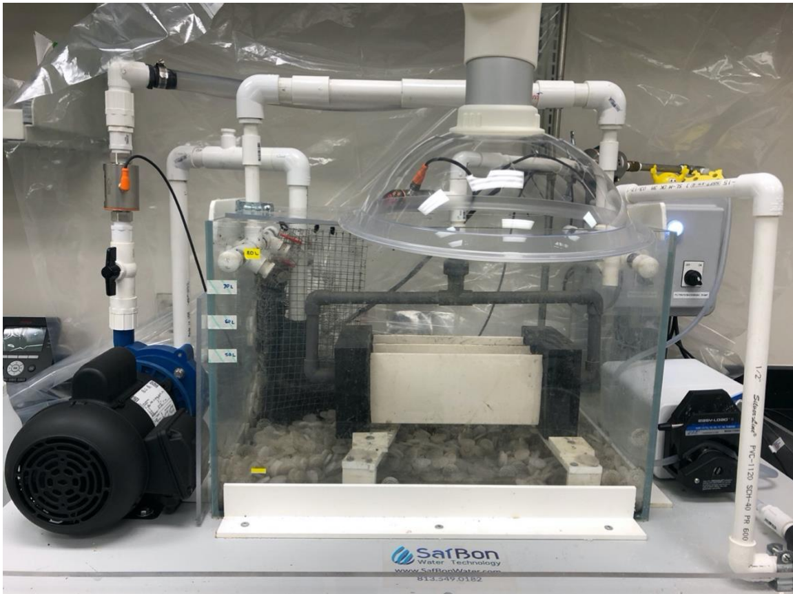
Figure 12. Photograph of the bench-scale AnBfMBR
