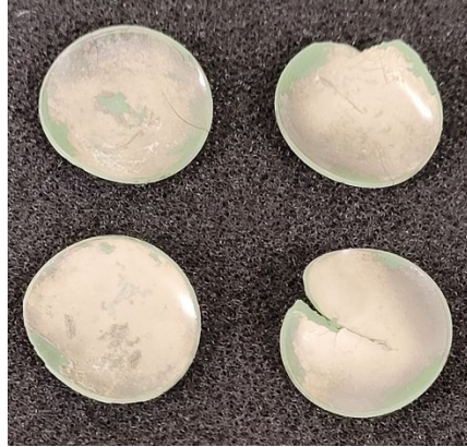
Figure 12: Double-Pressed SOFC Fabrication Attempt Results
