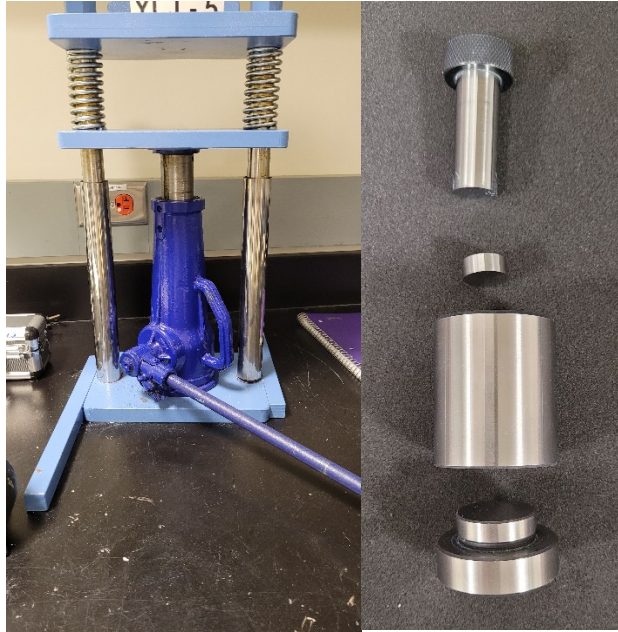
Figure 9: Dry Press and Dry Pressing Die Used to Create Ceramic Anode Discs
