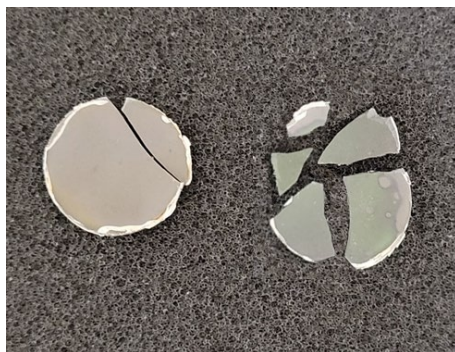
Figure 16: (1) SOFC Anode After Reduction, Before Siloxane Added to Fuel Source and (2) After L4 Siloxane Experiment
