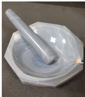
Figure 8: Mortar and Pestle Used for NiO+SDC Powder Mixing
