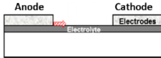
Figure 2: Cross-sectional diagram of a lateral PMC structure [4]
