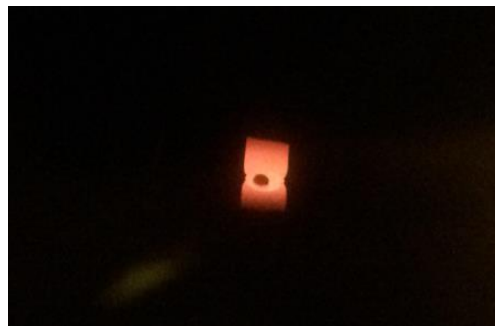
Figure 23: Hot resistive boat containing silver source shot
