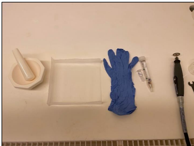
Figure 2.2 Tools for mechanical sample cleaning and preparation
