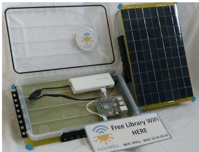
Figure 1: An image of two SolarSPELL Units (Theda, 2018). The unit on the left displays the inner components of the SolarSPELL unit, and the unit on the right displays a top view of the solar panel attached to each unit. There is a sign displaying the Wi-Fi signal name, as well as the web browser address that is used to access the library.
