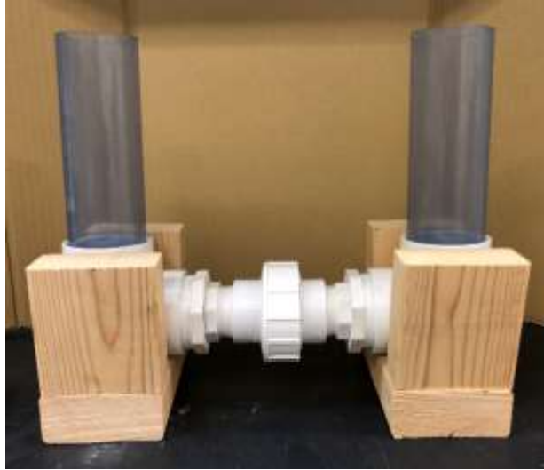
Figure B.1. Picture detailing the dead-end forward osmosis (FO) setup that was used for determination of urea transfer across the FO membrane.
