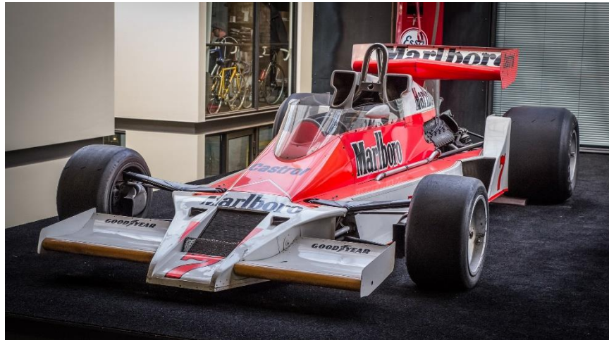
Figure 2: Endplates Added and Camber Increased in the 1970s (emkanicepic, 2019)
