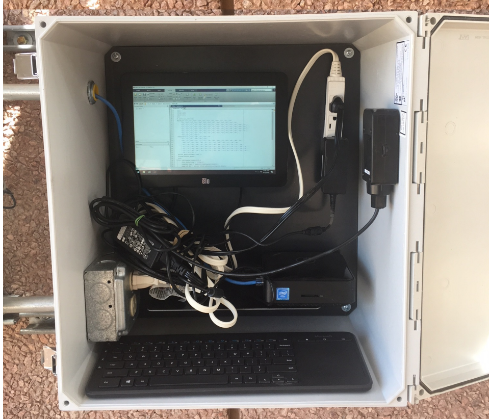
Figure A.3: The computer developed for controlling the 18kW solar array. This computer is connected to the transceiver which communicates to the SMDs and receives data.
