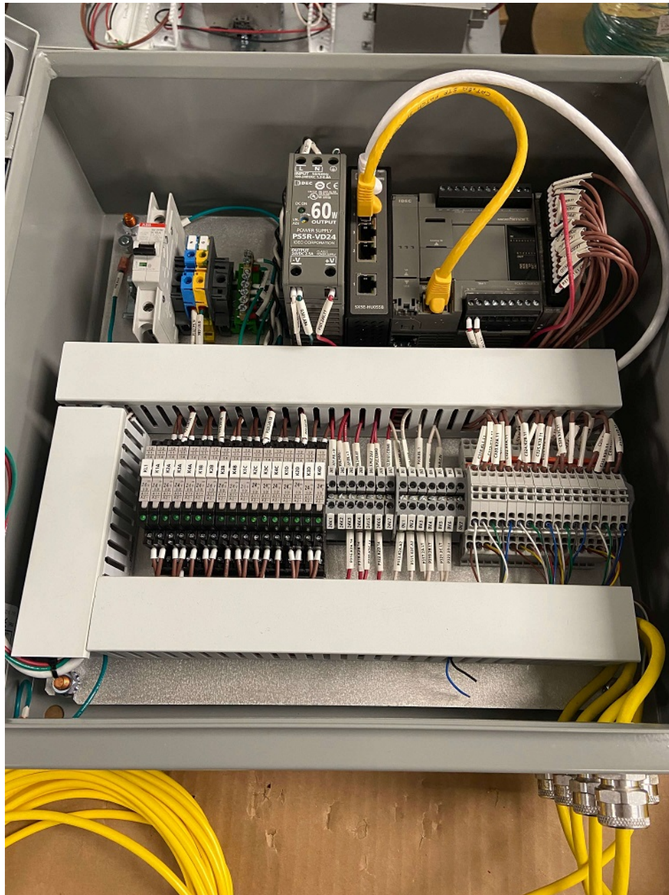
Figure 3.6: The MPP Tracking Is Controlled Automatically Through the Control Box Shown Here. The PLC Controls the Switches and Will Either Turn the Resistors on or off Depending on the Time of the Day.
