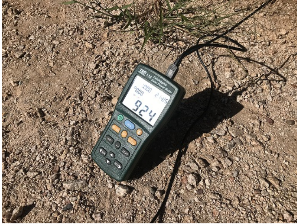
Figure A.7: The irradiance meter used to obtain irradiance measurements in real time. The irradiance meter has a sampling rate of 1s and it is placed on top of the PV module.
