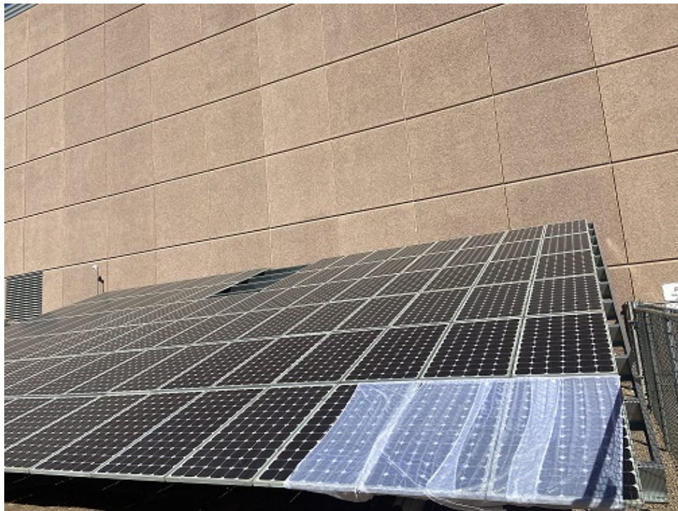
Figure A.9: An Example of a Simulated Shaded Module at ASU Research Park. This Corresponds to 25% Shading.
