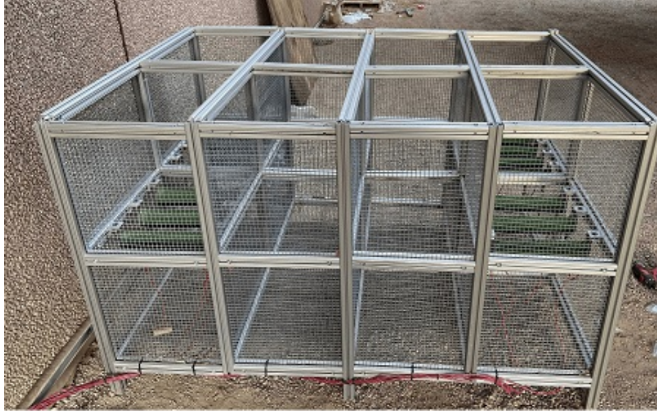
Figure 3.7: A Design of a 7 Resistor Load Bank. Four of the Resistors Are Always on and the Remaining Set of Resistors Turn on or off to Implement Various Conditions for Testing.
