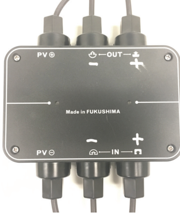
Figure 3.2: Smart Monitoring Device (SMD) Attached to a Solar Panel( Takehara and Takada (2013)).
